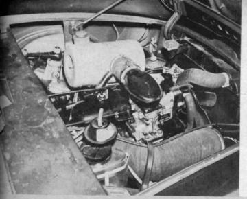
FIAT 1100 TV ENGINE, with its familiar Weber carburetor and ohv layout, is easily accessible, although the standard windshield washer, fresh air intake ducting, oil filter, etc. seem to crowd compartment. A well padded dash displays large side-by-side instrument dials with warning lights for low oil pressure and battery discharge.
